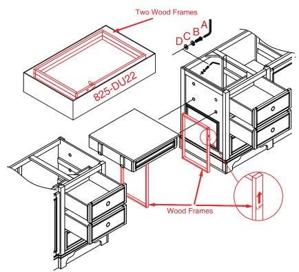
Step 3a: Locate the two rectangular wood frames included inside the carton. The frames are used to support the makeup drawer during assembly and make the installation process easier.
