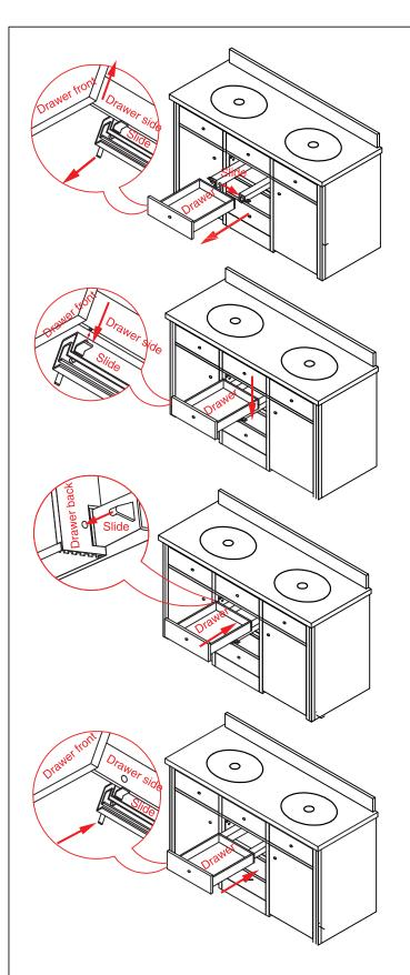
1. For removal, pull out the locking pin from the drawer side. Lift the drawer and pull it out from the cabinet.
